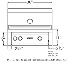
sides(rear or bottom access). Make these holes in the frame based on your requirements. 120V GFI outlet must be located within 6' of the 4" hole.
