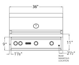
4" square holes for gas and electrical connections both left and right sides(rear or bottom access). Make these holes in the frame based on your requirements, 120V GFI outlet must be located within 6' of the 4" hole.
